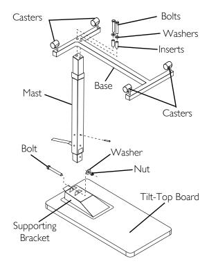
FIGURE 2 Assembling the Overbed Table - Model 6418
